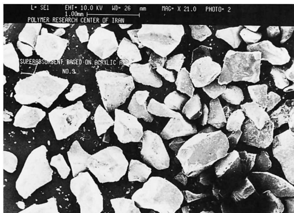
Figure 1 SEM of grounded superabsorbent without modification of particle size.
